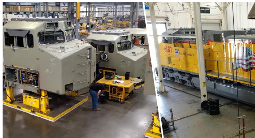
Left, a main cab for a Union Pacific modernized locomotive on the floor of Wabtec's Fort Worth, Texas, plant. Right, a modernized locomotive receives finishing touches.
