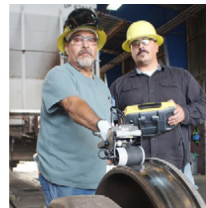
West Colton, California, Carman Welder John Moreno and Car Inspector Cesar Aguirre test a new wheel defect detector.
