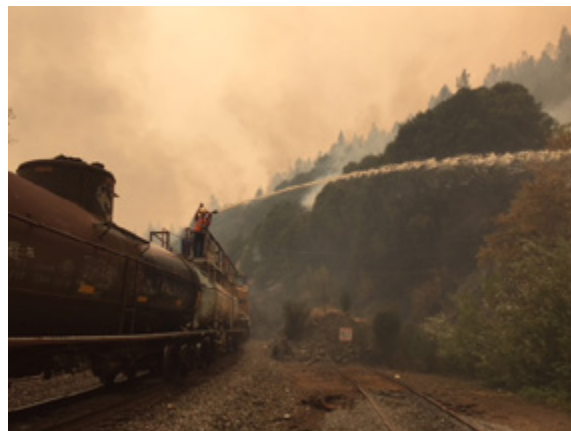
Northern California Service Unit employees between James and Pulga, California, use one of many "water cars" staged across the service unit to spray surrounding track.
