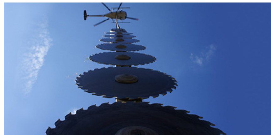
A 10-bladed saw suspended from a helicopter trims limbs and brush on rail rights of way.
