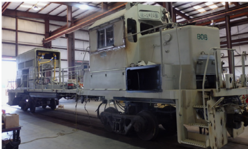
A stripped-down switcher locomotive waits to be repowered into a new Tier 4 switcher.
