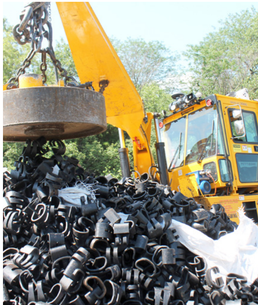
A speed swing operator compiles clips for recycling on the Marysville Subdivision in Nebraska.
