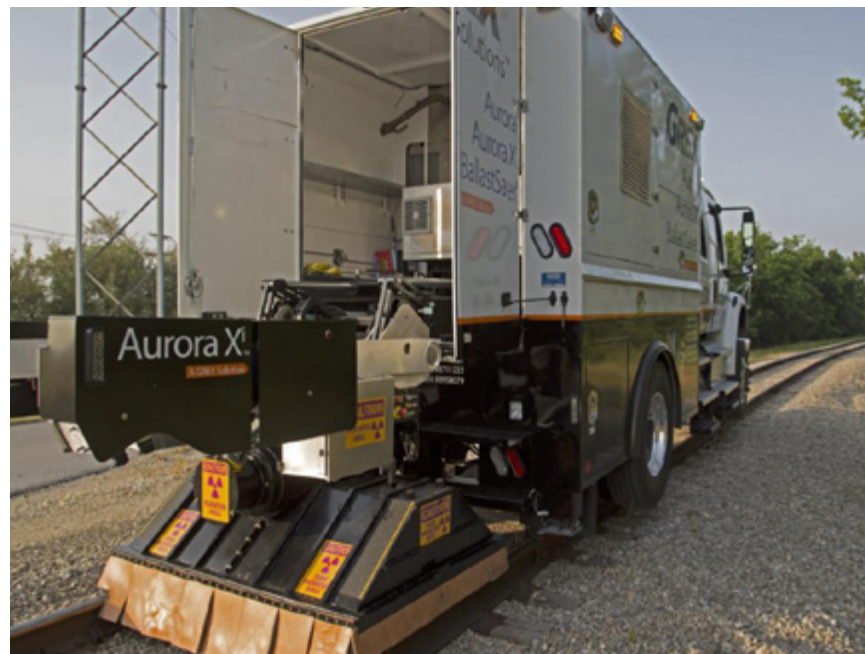
The Aurora system is used by track inspectors to examine rail tie quality.
